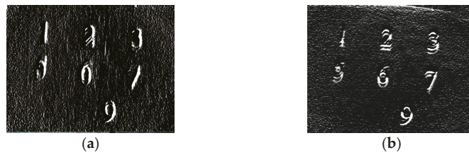
Figure 3. (a) Normalized Sobel gradient of the image along the x-axis; (b) normalized Sobel gradient of the image on the y-axis at 70 lux.
