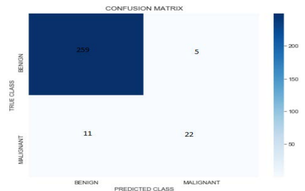
Fig. 6. A Confusion Matrix for the Two Classes – benign and Malignant Plotted against the True and Predicted Classes. Here, 259 Indicates TP, FP = 5, FN = 11 and TN = 22. The Ranking is shown for all the 297 Input Samples.
