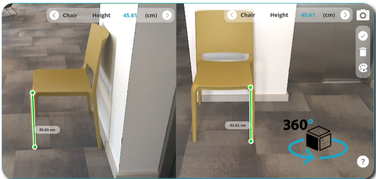
Fig. 7 A Change in POV of the device whereby 3D Measurement markers are fixed in Euclidian World-Coordinate space in accordance with the Time-of-Flight depth results
