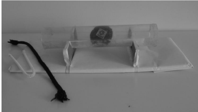
Figure 2. Narrow horizontal tube containing pom-pom (with sticker attached), bent pipe cleaner and string.
