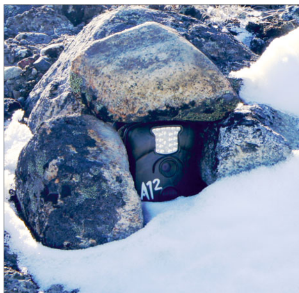
Fig. 2. Example of a trail camera installation at the lake shore.
