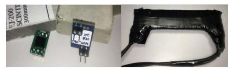
Figure 1. Left) Example of raw and polished EJ-200 plastic scintillator bars and two commercial SiPM boards. Right) The scintillator is equipped with SiPMs and wrapped with black tape to avoid external stray photons.
